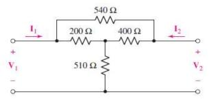
b) Obtain a complete set of h parameters which describe 6 M the two-port network as shown below.
