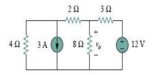
b) Compute the voltage across each resistor in the 6 M following figure.
